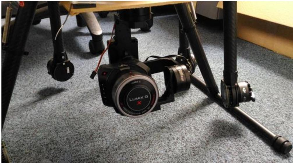
**Fig 3.3: Camera and Gimbal on a temporary support.**
