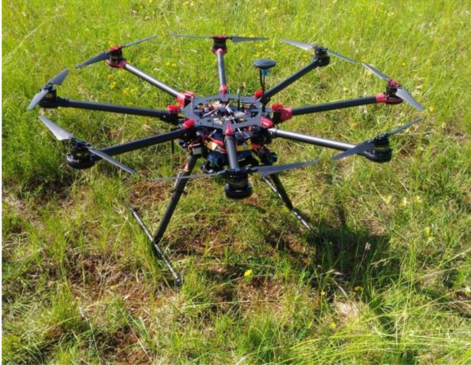
**Fig. 3.1: Drone platform with the drone core components (without flight nor audiovisual payload), ready for basic flight tests.**
